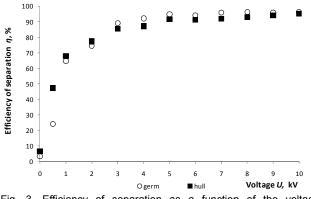
Fig. 3. Efficiency of separation as a function of the voltage supplying the bifilar winding
