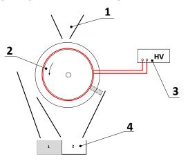
Fig. 2. Electroseparator model: 1 - material feeder, 2 - electric separator with bifilar winding, 3 - HV power supply, 4 - container divided into 2 chambers
