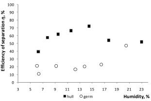
Fig. 4. Efficiency of separation as a function of humidity
