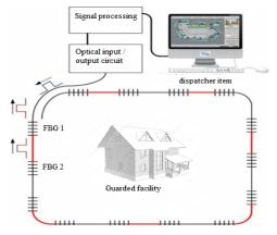
Fig.3. The principle of operation of a fiber-optic security system based on Bragg gratings
