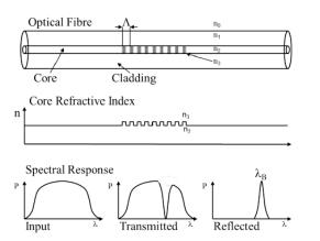
Fig.1. The principle of operation of FBG
