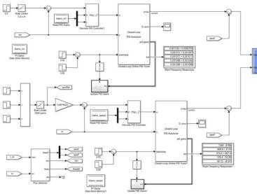
Fig. 4. Simulation model for control system of induction motor's inverter
