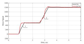
Fig. 5. Simulation results for motor speed: 1 - FOC; 2 - NN FOC
