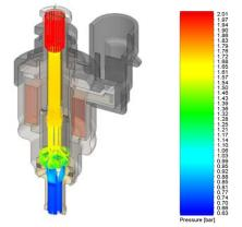
Fig.1. Gas flow trajectory through the injector (longitudinal section view)
