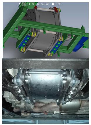
Fig.8. Design (3D model) of the drive mounting in the VW Touareg and below the final result of the work in a mechanical workshop
