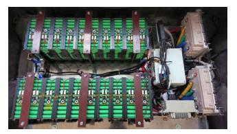
Fig.9. The battery pack installed in the vehicle with engine controllers
