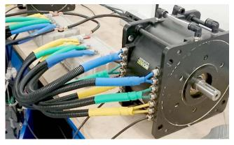
Fig.7. View of the test stand: with a BLDC motor (HPM-20 kW) powered from the converter
