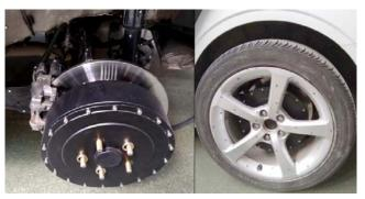
Fig.6. The way of mounting the BLDC drive in the rear wheel hub - Audi A3  $\,$
