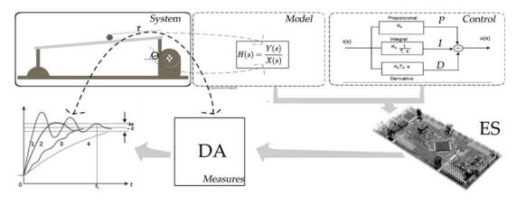
Fig. 4. Ball and Beam HIL simulation
