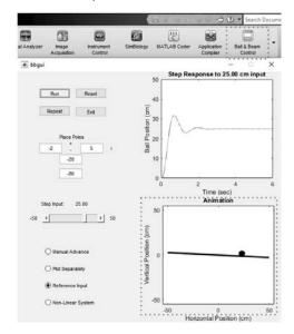
Fig. 3. Ball and Beam simulation. In the app "Ball & Beam Control", that can be downloaded and installed online, it is possible to adjust the control gains, the initial values and the set-points, in addition to the animation of the system.
