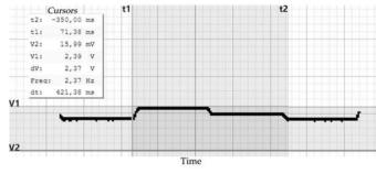
Fig. 14. Capacitor output voltage for the SFL control of the SEPIC converter - HIL simulation. Note: 0.1 s / div on the x axis; on the y axis a 2.4 V in DA converter corresponds to 16V of the real voltage.
