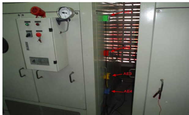
Fig. 10. The location of the vertical signal sensor installation.
