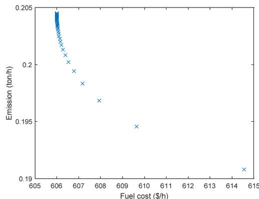
Fig. 3. Fuel cost and emission optimization with MOALO (Case A)
