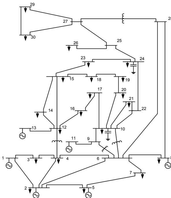
Fig. 1. Single-line diagram of IEEE 30-bus test system [20]
