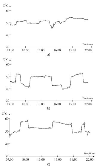
Fig. 1. The graphs of changes in the controlled parameters when setting and stabilizing the temperature of the heat flow of the Wilo TOP S 50/10 pump with VLT Micro Drive FC-51: a) setting parameter change with AMA function; b) setting parameter change without AMA function; c) preservation of original parameters with AMA function (dashed line – setting the parameter, solid line – the results of its processing)
