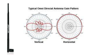
Fig.2. TL-ANT 2408CL omni-directional microwave-band antenna gain pattern.
