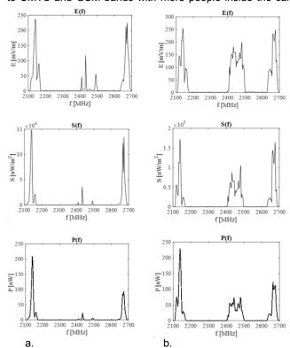
Fig.3. Measured values in CAR1 a.) turn off mobile phone. and b.) during phone call
