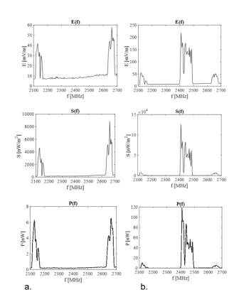
Fig.4. Measured values in CAR2 a.) turn off mobile phone. b.) during phone call
