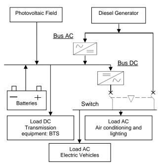
Fig.3. Hybrid system topology
