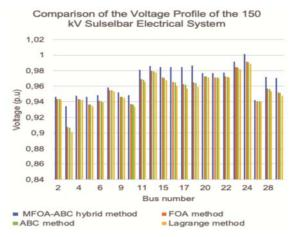
Fig.5. Comparison graph of the voltage profile by using MFOA-ABC hybrid method with other methods
