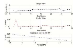
Fig.6. Graph of the V-P curve by using the MFOA-ABC hybrid optimization method with loading on bus 3 of 289  $\rm MW$
