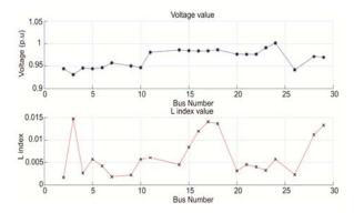
Fig.4. The L index value and voltage of the 150 kV Sulselbar real system using the Hybrid MFOA-ABC method
