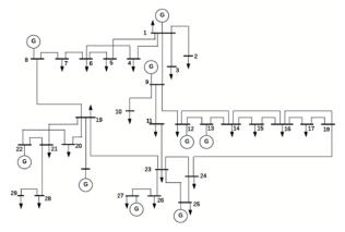
Fig.1. Single line diagram of the 150 kV Sulselbar electrical system
