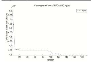
Fig.7. The convergence curve of generating fuel costs  $\,$  by using MFOA-ABC hybrid method when loading on bus 3 of 289 MW  $\,$
