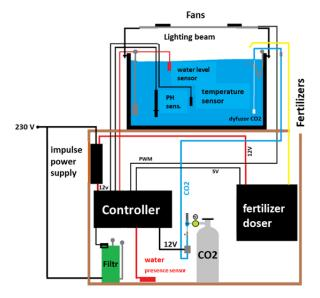
Fig. 4. Block diagram of an aquarium controller programmed in the Arduino environment
