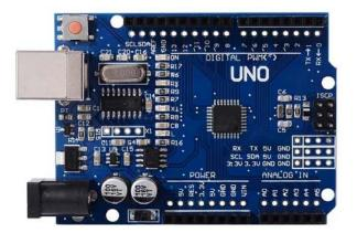
Fig. 3. The Arduino Uno microcontroller used in the aquarium controller model [5].
