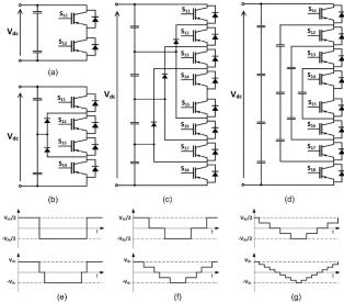
Fig. 1. One leg (phase) diagram of inverter a) two-level, b) threelevel, c) five-level NPC, d) five-level FC, e) phase voltage (upper) and line-to-line voltage (lower) of two-level inverter, f) phase voltage (upper) and line-to-line voltage (lower) of three-level inverter, g) phase voltage (upper) and line-to-line voltage (lower) of five-level inverter
