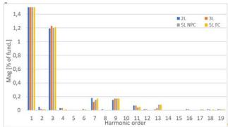
Fig. 5. FFT analysis of current harmonics
