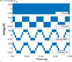
Fig. 4. Phase voltage comparison for different types of multilevel inverters
