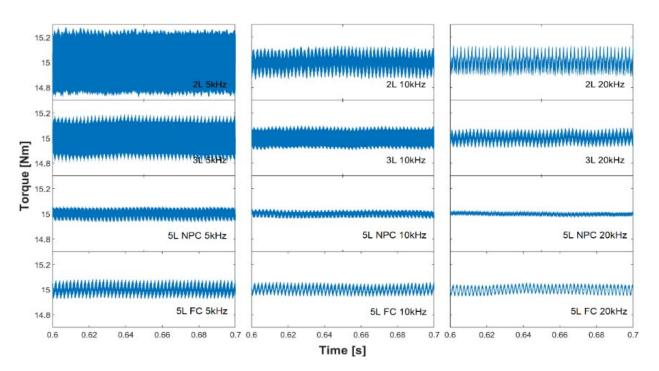
Fig. 8. Torque comparison for different types of multilevel inverters and switching frequencies
