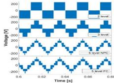
Fig. 3. Line-to-line voltage comparison for different types of multilevel inverters
