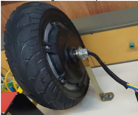
Fig.10. Outrunner BLDC motor, 36 V/350 W
