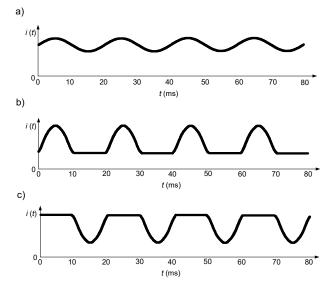
Fig.1. Simplified earth fault current waveforms i(t) in case of the earth fault on the DC side in a PV installation; according to [12]. Waveforms containing: a) sinusoidal component and smooth DC, b) pulsating DC (half-wave) and smooth DC (both components of the same polarity), c) pulsating DC (half-wave) and smooth DC (components with opposite polarity)
