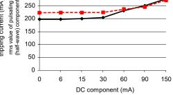
Fig.4. The tripping current of two A-type RCDs of  $I_{\Delta n}$  = 300 mA (RCD4, RCD5) under the residual test current composed of: a) AC sinusoidal and smooth DC components, b) pulsating (half-wave) and smooth DC components. The smooth DC component has the following values: 0, 6, 15, 30, 60, 90, 150 mA
