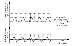
Fig.6. Oscillogram of the primary current (half-wave) of the RCD's current transformer and oscillogram of its induced secondary voltage. No smooth DC component superimposed on the halfwave. Current transformer from an RCD of A-type and  $I_{An}$  = 300 mA
