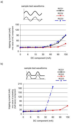
Fig.3. The tripping current of three A-type RCDs of  $I_{\Delta n}$  = 30 mA (RCD1, RCD2, RCD3) under the residual test current composed of: a) AC sinusoidal and smooth DC components, b) pulsating (half-wave) and smooth DC components. The smooth DC component has the following values: 0, 6, 15, 30, 60, 90, 150 mA
