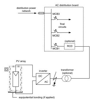
Fig.2. Sample installation with PV energy sources. RCD – residual current device, MCB – miniature circuit-breaker
