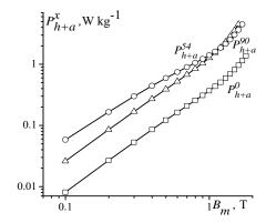
Fig. 2. Directional curves of a sum of  $P_h$  and  $P_{ex}$  components of ES grade M150-35S [13]
