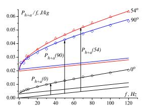
Fig. 1. Energy loss per unit mass versus frequency for different magnetizing directions obtained for steel grade M150-35S at  $B_p$  = 1.2 T
