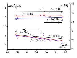
Fig. 5. Parameters *m* and *x*(50) of Eq. (4) as a function of specific total loss anisotropy  $\Delta P_S^{99.0}$  and frequency *f*
