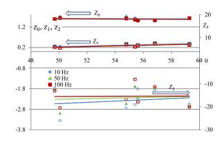
Fig. 6. Parameters  $z_0, z_1$  and  $z_2$  of (5) as a function of anisotropy  $\varDelta P_S^{090}$  and frequency
