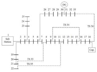
Fig. 1. Network Reconfiguration by installation of DGs and Capacitor in 33-node test system
