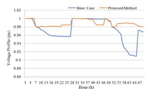
Fig. 6.Voltage profile for base case and Reconfiguration with placement of DG and capacitor in 69-bus test system
