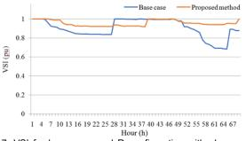
Fig. 7. VSI for base case and Reconfiguration with placement of DG and capacitor in 69-bus test system
