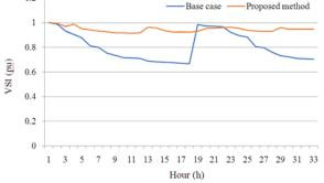
Fig. 3. VSI for base case and Reconfiguration with installation of DG and capacitor in 33node test system
