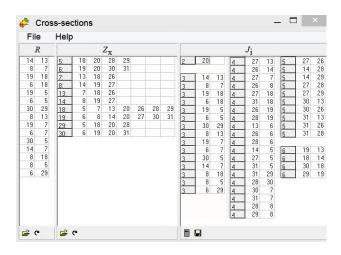
Fig.4. Computer program for the formation of minimal crosssections (minimal-cut failure states)  $[J_i]\theta$ : i = 2, 3, 4, 5, 6
