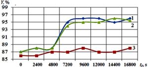
Fig. 6. Germination of the resulting grain raw material depending on the concentration of ozone: 1 - at ozone concentration  $10 \text{ mg/m}^3$ ; 2 - at ozone concentration  $15 \text{ mg/m}^3$ ; 3 - in the absence of ozone in the composition of the drying agent.
