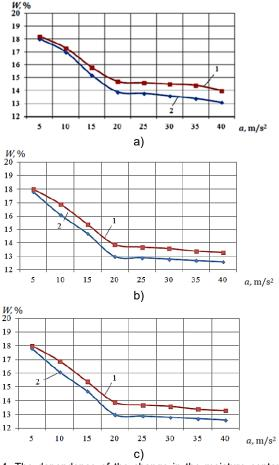
Fig. 4. The dependence of the change in the moisture content of grain raw materials depending on the vibration acceleration: a - at drying agent temperature 45 °C; b - at drying agent temperature 55 °C; c - at drying agent temperature 65 °C; 1 - at the technological loading of the drying chamber 75% from total volume; 2 - at the technological loading of the drying chamber 50% from total volume.
