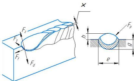
Fig. 1. The power balance of the melt bath:  $F_z$  – the force acting on the front of the melt;  $F_z$  – the displacement force of the liquid metal;  $F_t$  – tangential forces in the melt bath, due to the movement of the electrode;  $F_d$  – force of electric arc;  $F_p$  – surface tension forces during solidification of liquid metal
