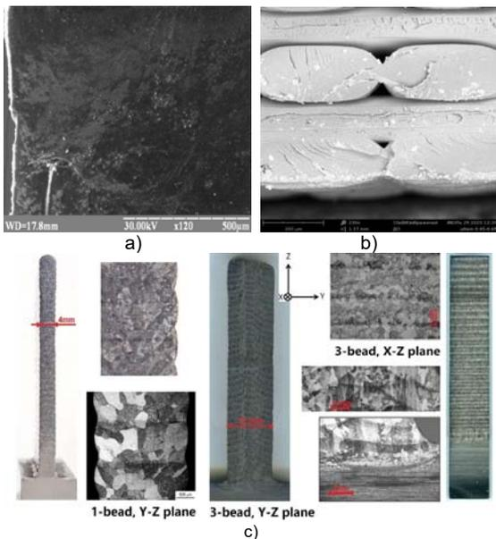
Fig. 4 Comparison of end sections of model fragments obtained by surfacing (a), FDM-printing with plastic (b) and additive technology xBeam 3D Metal Printing (c). Microphoto (b) – ULTEM 9085 plastic, element created on the STRATASys FORTUS 380 printer. Cavities and defects of the open end face are observed on the sections
