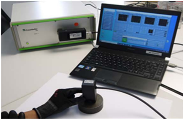
Fig.1. 3MA NDT system under inspection
