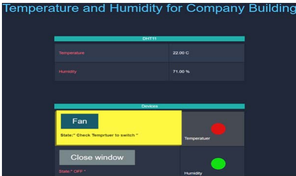
Fig. 6. Illustrated temperature when above the set value
