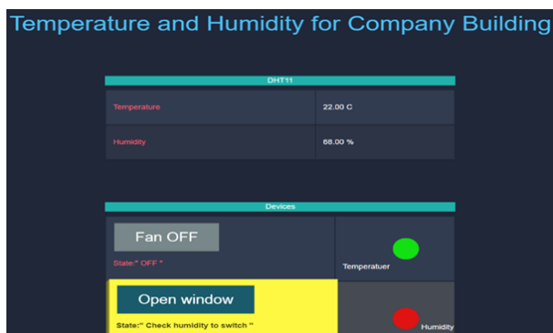
Fig. 7. Illustrated humidity when condition above the set value
