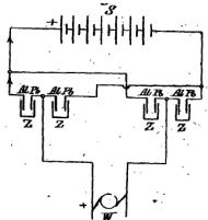
Fig.4. The bridge circuit of a 1-phase electrolytic rectifier included in the British patent specification obtained by Charles Pollak [13]: W - alternating voltage source; Z – electrolytic cell with Al and Pb electrodes; S - accumulator battery
