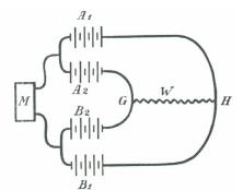
Fig.6. Bridge circuit of a 1-phase electrolytic rectifier developed by prof. Leo Graetz [16]: *M* - alternating voltage source; W - receiver powered by rectified voltage; A1, A2, B1, B2 - electrolytic rectifier cells
