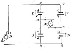
Fig. 5. The bridge circuit of a 1-phase electrolytic rectifier, included in the description of the American patent obtained by Charles Pollak [15]: D - alternating voltage source; M - receiver powered by rectified voltage; p, q, r, s - the cells of the electrolytic rectifier (marked with the symbols used for electrochemical cells)
