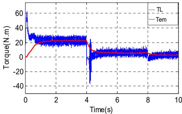
Fig. 11. Electromagnetic and load torque
