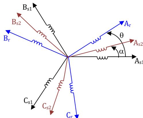
Fig.4. Windings of the double star induction motor
