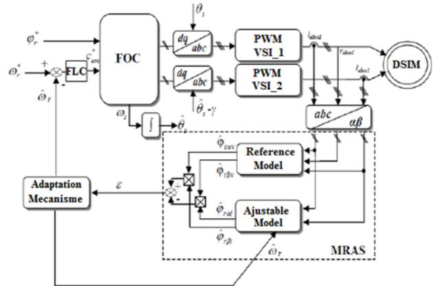
Fig.9. Fuzzy speed sensorless control of field-oriented DSIM with MRAS observer
