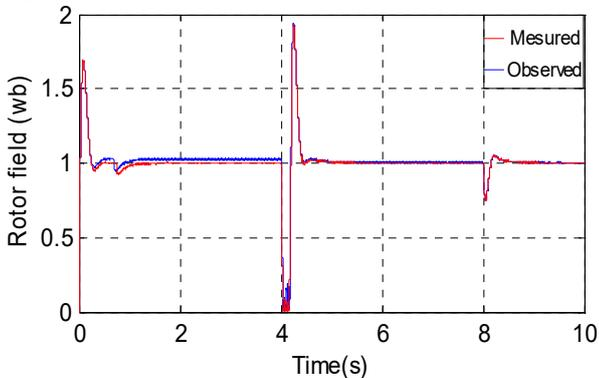
Fig. 13. Measured and observed rotor field
