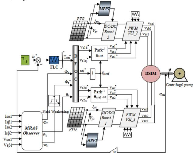
Fig.1. Schematic diagram of proposed solar water pumping system
