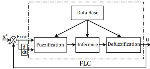
Fig.7. Fuzzy controller structure
