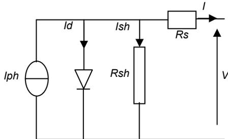
Fig.2. Equivalent circuit of a PV module
