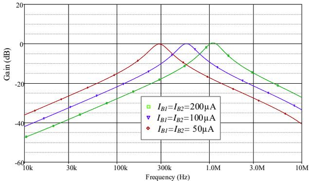
Fig.7. Bandpass responses by changing the bias currents  $I_{B1} = I_{B2}$
