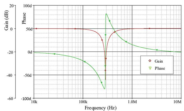
Fig.5. shows gain response of proposed circuit output-current gain of the LP, BP, AP,HP and BR
