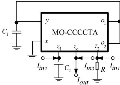
Fig.3. Proposed filter of MO-CCCCTA
