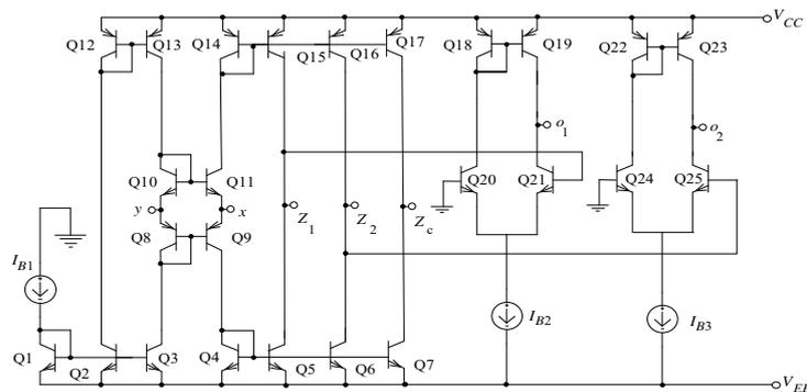
Fig.2. Internal Construction of MO-CCCCTA
