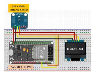
Fig.2 Schematic circuit of the hardware device
