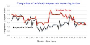
Fig. 4 The calibration test between the proposed IoT device and the standard one
