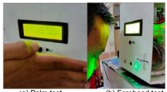
(a) Palm test (b) Forehead test Fig. 5 The temperature test of the body parts measured by the proposed prototype
