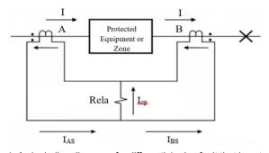
Fig.1. A single-line diagram of a differential relay fault that is out of zone.
