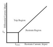
Fig.3. Differential relay characteristics.
