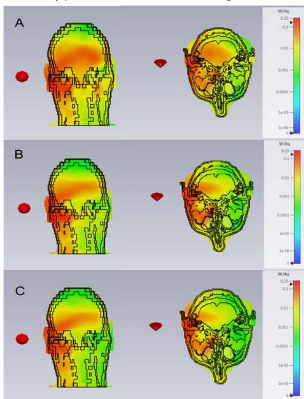
Fig.4. Numerical simulation showing SAR<sub>10</sub> spatial distribution at the head cross-section in the vertical direction and horizontal direction for the frequency 825 MHz (A), 1760 MHz (B) and 2109 MHz (C).
