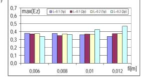
Fig.6. The influence of the diameter of the reinforcement on the max( $E_z$ ) value with the conductivity  $\sigma$ =0.01 S/m and the relative electric permittivity: (a)  $\varepsilon_r$ '=5; (b)  $\varepsilon_r$ '=6; (c)  $\varepsilon_r$ '=7; (d)  $\varepsilon_r$ '=8
