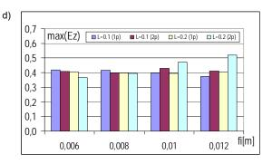
Fig.5. The influence of the diameter of the reinforcement on the max( $E_z$ ) value with the conductivity  $\sigma$  =0.004 S/m and the relative electric permittivity : (a)  $\varepsilon_r$ '=5; (b)  $\varepsilon_r$ '=6; (c)  $\varepsilon_r$ '=7; (d)  $\varepsilon_r$ '=8
