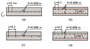
Fig.3. Variants of the analysed walls: (a) L10(1p); (b) L10(2p); (c) L20(1p); (d) L20(2p)
