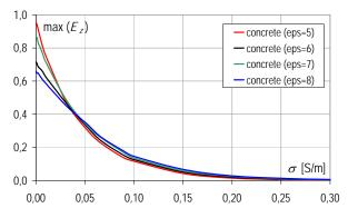
Fig.1. Changes in the  $max(E_z)$  value depending on the conductivity for different values of relative dielectric permittivity
