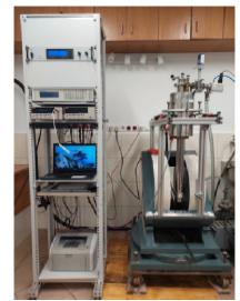
Fig. 2. Low temperature cryostat with control unit
