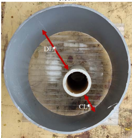
Fig. 4. Convergent Length (CL)= 2.5cm, Divergent Length (DL)= 5.5cm
