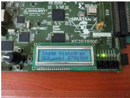
Fig. 10: number of clock cycles needed to implement parallel histogram with drawing figures (Image and Histogram)
