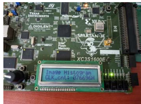
Fig. 8: number of clock cycles needed to implement serial histogram with drawing figures (Image and Histogram)
