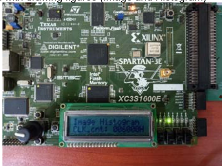
Fig. 11: number of clock cycles needed to implement parallel histogram without drawing figures
