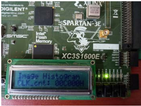
Fig. 9: number of clock cycles needed to implement serial histogram without drawing figures
