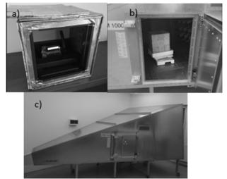
Fig. 5. Test stand: a) small test chamber made of composite plates, b) the chamber placed in GTEM1000 chamber, c) GTEM1000 chamber.
