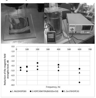
Fig.3. Shielding of composites for frequencies <1 kHz, a) view of the transmitting coil, b) view of the measuring station, c) shielding level in the frequency range 40-600 Hz for three examples.
