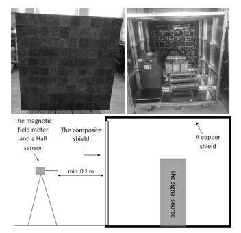
Fig. 6. The large test chamber: (a) composite screen view, (b) interior view, (c) diagram of the stand for measuring the magnetic field induction  $f = 50 \, \text{Hz}$  at a distance of 0.1 m from the chamber wall with and without a composite screen.
