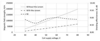
Fig. 7. 50 Hz field shielding effectiveness.
