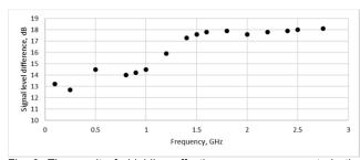
Fig. 8. The result of shielding effectiveness measurements in the range 0.2 - 2.75 GHz.
