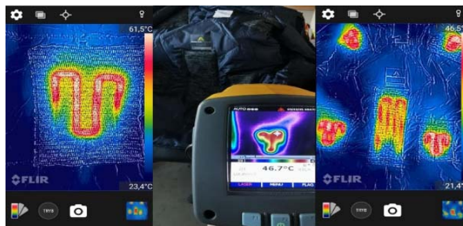
Fig.7. Temperature measurement of heating mats using thermal imaging.
