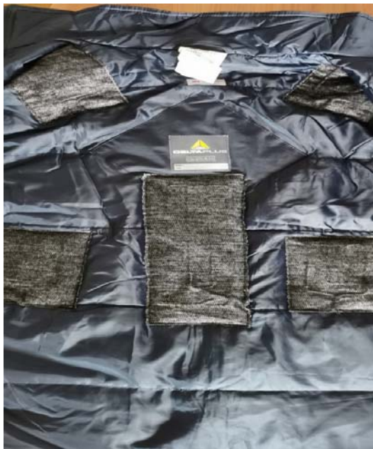
Fig. 4. Carbon fiber heating mats sewn into the jacket.
