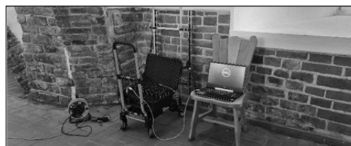
Fig.1. The measuring station equipped with an electric tomograph and two metal strips with 16 electrodes each
