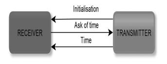
Fig. 3. Method of measuring distance by measuring the response time
