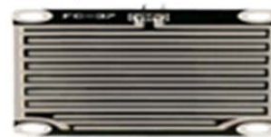
Fig.7. The Rain Detector (Sensor)
