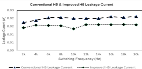
Fig. 8. Conventional H5 and Improved H5 Leakage Current
