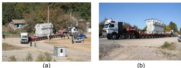
Fig.3. Transportation of a power transformer for commissioning at a power plant in wartime conditions in Ukraine.
