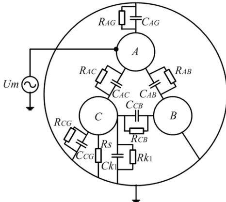
Fig.2. Modified inspection scheme of a three-core power cable:  $C_k$  – electrical capacitance of an auxiliary reference capacitor,  $R_k$  – shunt resistance, caused by dielectric power losses in the reference capacitor,  $R_s$  – auxiliary variable resistor.
