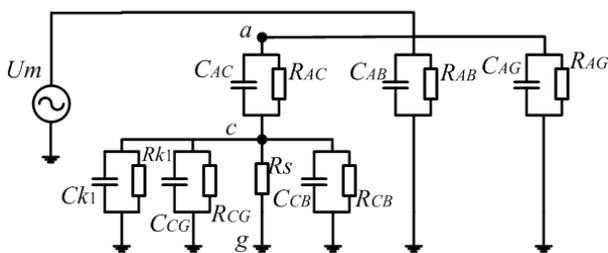
Fig.3. Expanded form of the modified inspection scheme presented in Fig.2
