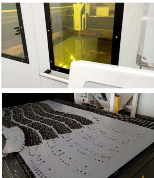
Fig.1. Laser cutting of Permanent magnet synchronous motor magnetic sheets. Photo courtesy of Kisielewski sp z.o.o.
