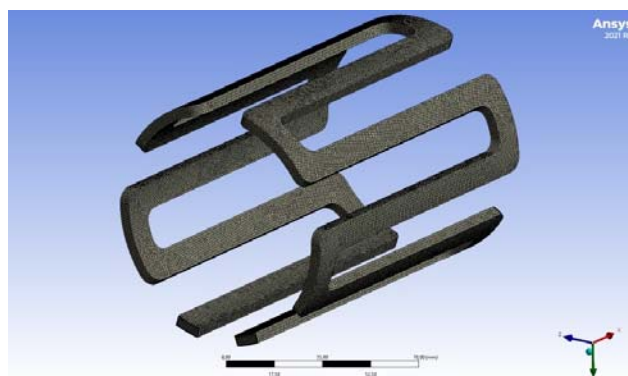
Fig.5. Coolant with a finite element mesh in ANSYS software
