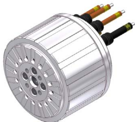
Fig.3. CAD model of an induction motor with an external rotor
