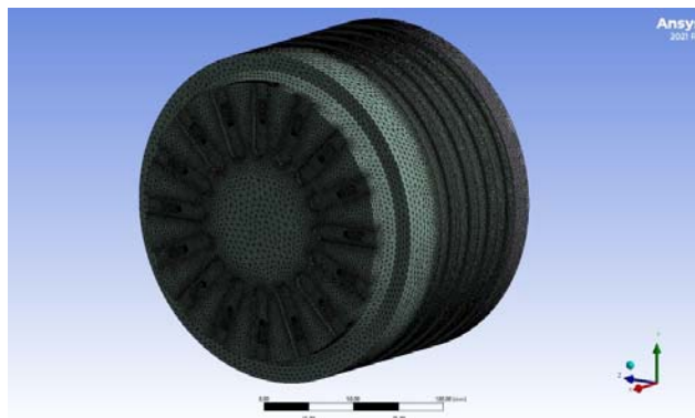
Fig.4. Motor model with a finite element mesh in ANSYS software
