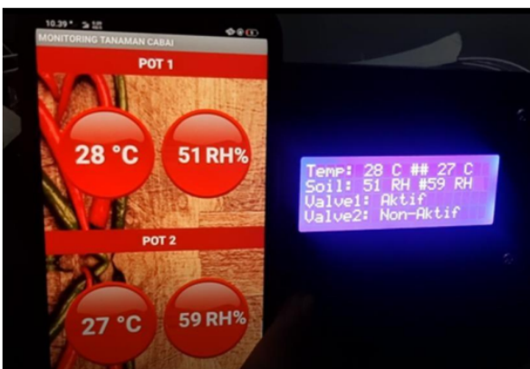
Fig 12. System Monitoring Display for each Crop
