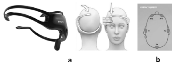
Fig. 1. a - Emotiv Insight neurohelmet, b - electrode arrangement diagram on the head, Source: https://www.emotiv.com/epoc-flex/
