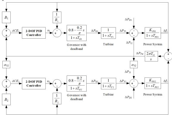
Fig.1. Transfer function model of interconnected two-area thermal system with governor dead band
