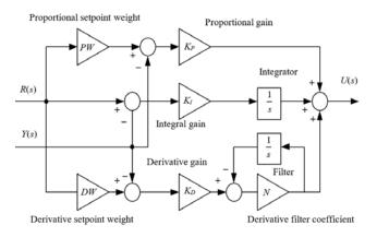
Fig.2. Two degrees of freedom (2-DOF) PIDcontroller
