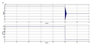
Fig. 8. Voltage and current waveforms vstime at MOV1.
