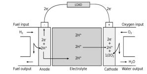
Fig.1. Fuel cell principle [4]
