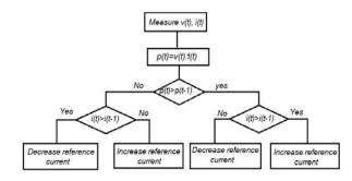
Fig. 10 Perturb and observe (P&O) MPPT algorithm
