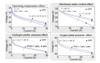
Fig. 6 Operating parameters effect on fuel cell polarization curve and maximum power point
