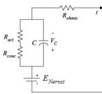
Fig.2. PEMFC Equivalent dynamic electrical circuit
