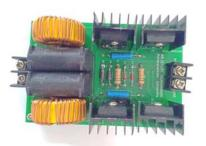
Fig.4. The LC oscillator does without the Caprio technique with the prototype circuit board.
