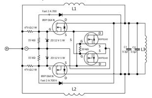
Fig.3. The LC oscillator does without the Caprio technique with the prototype circuit board.
