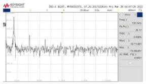
Fig.11.The frequency of the LC oscillator with the caprio technique, number of inductance turns L3 = 17  $\,$
