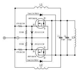
Fig.1. The LC oscillator without the Caprio technique.
