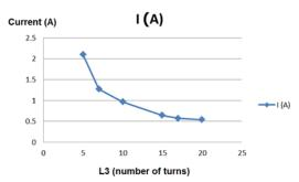
Fig.13. The current of the LC oscillator using the caprio technique when varying L3  $\,$
