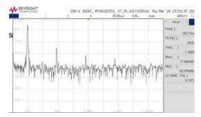
Fig.9. The frequency of the LC oscillator with the caprio technique, number of inductance L3 = 10 turns.
