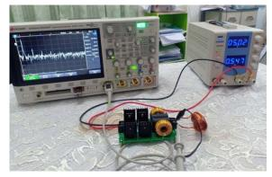
Fig.6. Frequency and THD measurements of the LC oscillator using the Caprio technique.
