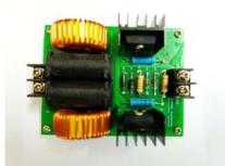
Fig.2. The LC oscillator does without the Caprio technique with the prototype circuit board.
