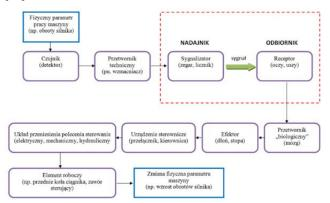
Fig. 1. The information chain and its relationship to the control process [8].
