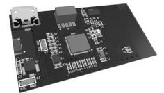
Fig. 3. WiFi transducer integrated circuit
