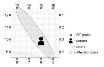
Fig. 1. RF sensor network with elliptical weight model
